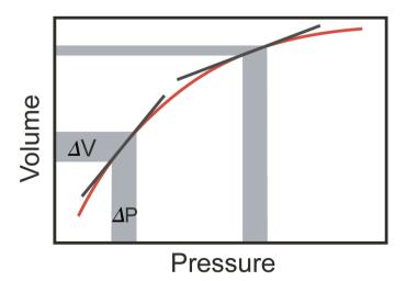
**FIGURE 1** Compliance curve for a biological tissue such as an artery. At low pressures and volumes, compliance (slope of tangent) is much greater than at high pressures and volumes. The change in volume ( $\Delta V$ ) for a given change in pressure ( $\Delta P$ ) is greater at higher compliance (C) because C =  $\Delta V/\Delta P$ .
