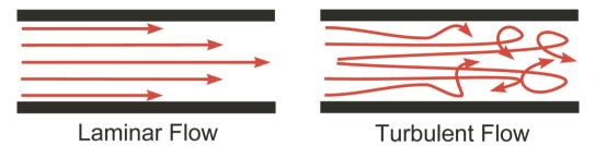
**FIGURE 1** Laminar versus turbulent flow. In laminar flow, blood flows smoothly in concentric layers parallel with the axis of the blood vessel, with the highest velocity in the center of the vessel and the lowest velocity next to the endothelial lining of the vessel. When laminar flow becomes disrupted and turbulent, blood no longer flows in layers, but rather moves in different paths, often forming vortices.
