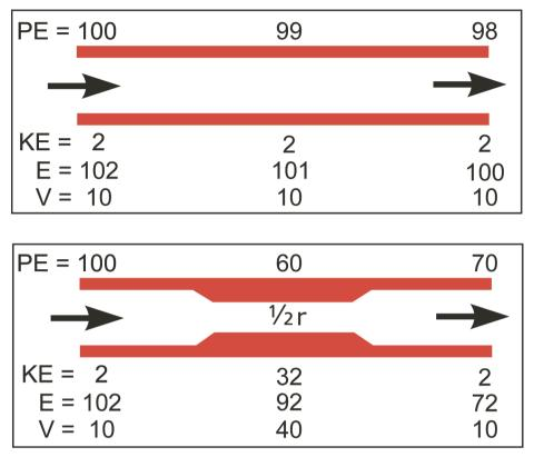
**FIGURE 1** Effects of vessel narrowing (stenosis) on energetics of flow. Vessel narrowing (stenosis) increases velocity (*V*) and kinetic energy (*KE*), and decreases pressure (potential) energy (*PE*) and total energy (*E*). The following relationships are illustrated in this figure: E = KE + PE;  $KE \propto V^2$ ;  $V \propto 1/r^2$ .
